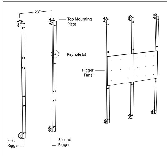
Start by mounting the first Rigger on the wall in it's planned location. Fasten the Rigger with a single screw through the top mounting plate and use a level to insure that the Rigger is straight. Fasten the rest of the screws to firmly mount the Rigger on the wall.
